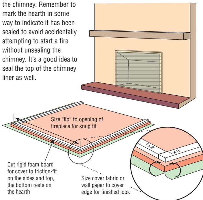
*A friction-fit fireplace cover can be fabricated out of rigid foam board, 1x2 lumber, glue and a covering that can be fabric or a material to suit the decor.*
