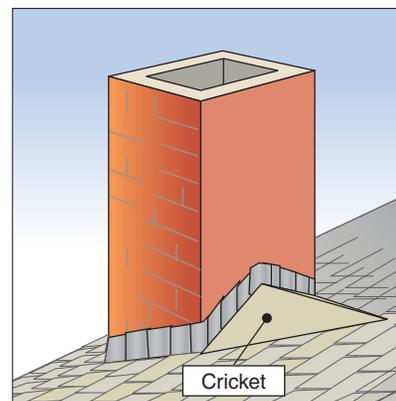
*A cricket helps divert roof runoff away from the chimney*
