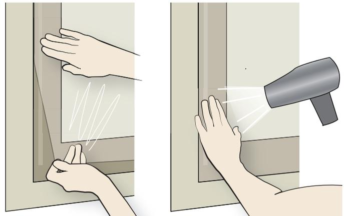
Shrink wrap plastic "storm" window coverings are a low cost, short-term solution to sealing a leaky window.
